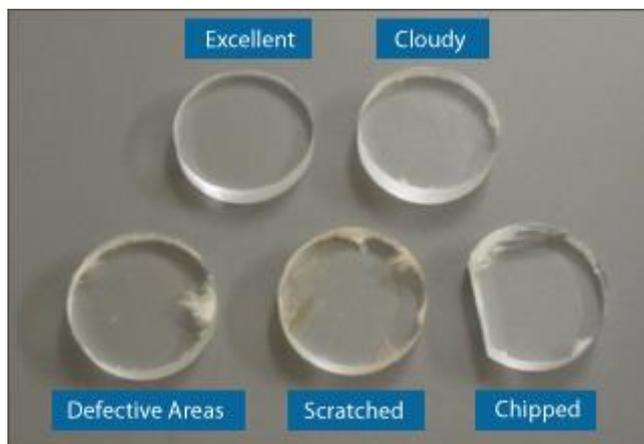
Figure 19: Sodium chloride (NaCl) plates in various conditions.
