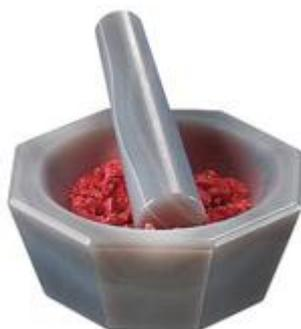
Figure 23: Agate mortar and pestle. Image reproduced with permission from Cole-Parmer (Hanwell, London, UK).
