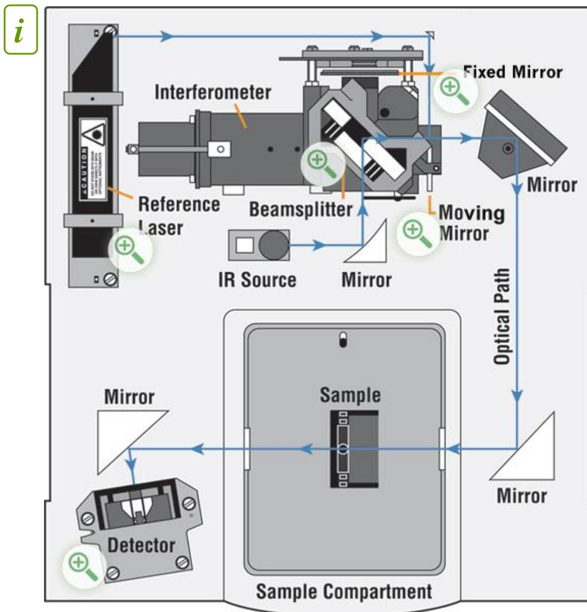
Figure 15: Operational Schematic of a Thermo Nicolet FTIR Instrument. Image reproduced with permission from Thermo Fisher Scientific (Madison, WI, USA).
