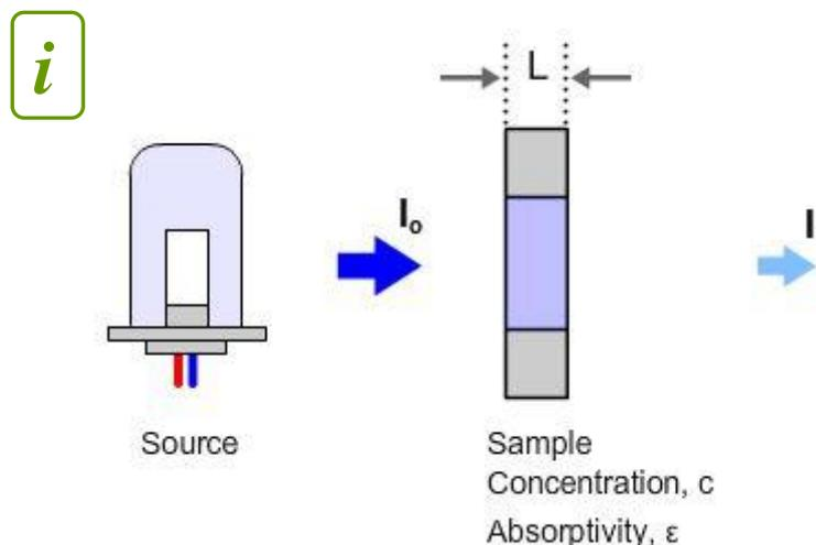
Figure 10: Absorption of infrared radiation of radiant power  $I_0$ . The radiation leaving the sample has radiant power  $I$ .
