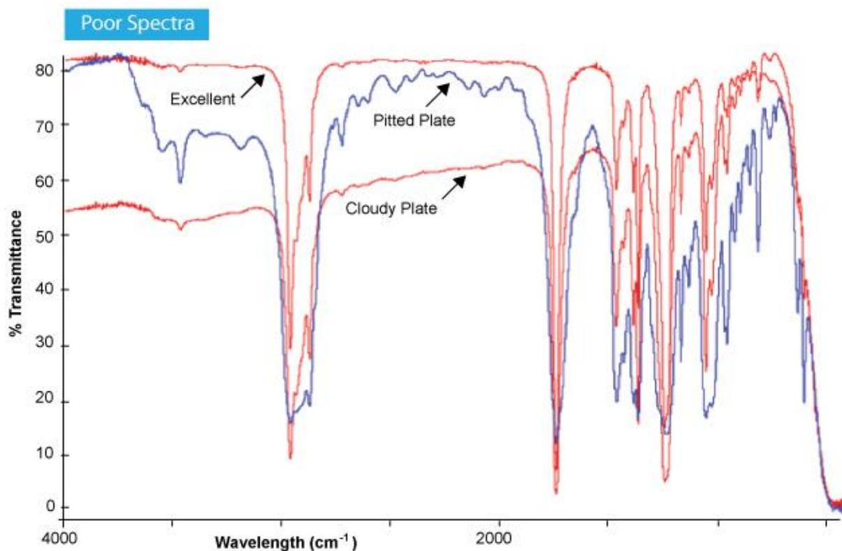
Figure 20: Representative spectra obtained with sodium chloride (NaCl) plates in various conditions.
