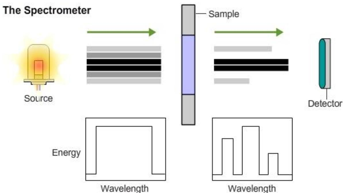
Figure 11: Sample absorption of IR radiation.
