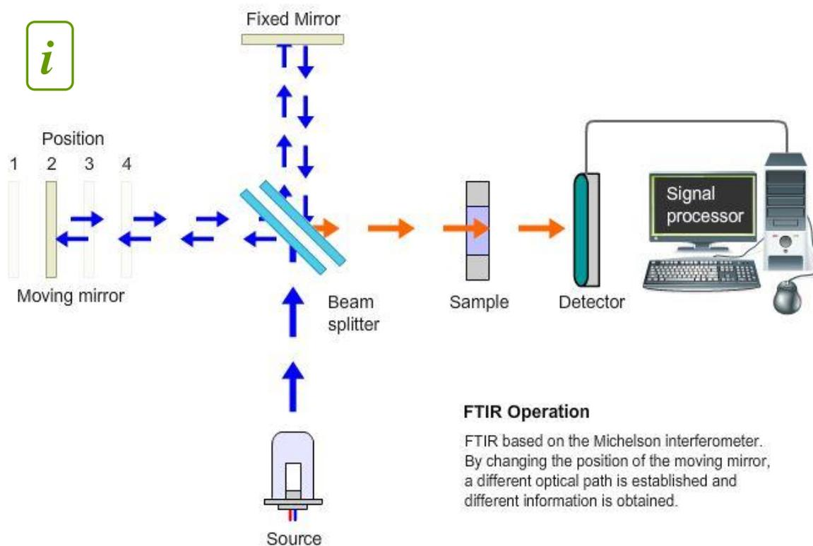
Figure 16: FTIR based on the Michelson interferometer. By changing the position of the moving mirror, a different optical path is established and different information is obtained.
