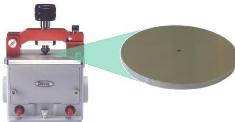
Figure 26: ATR Instrument. Image reproduced with permission from Specac (Orpington, Kent, UK).
