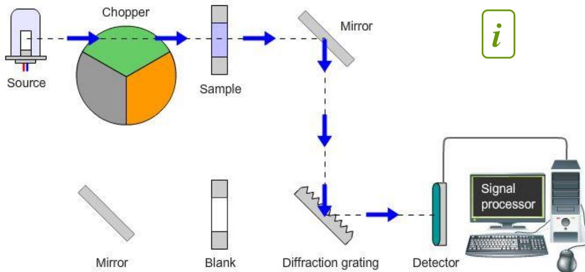
Figure 14: The double beam IR instrument.
